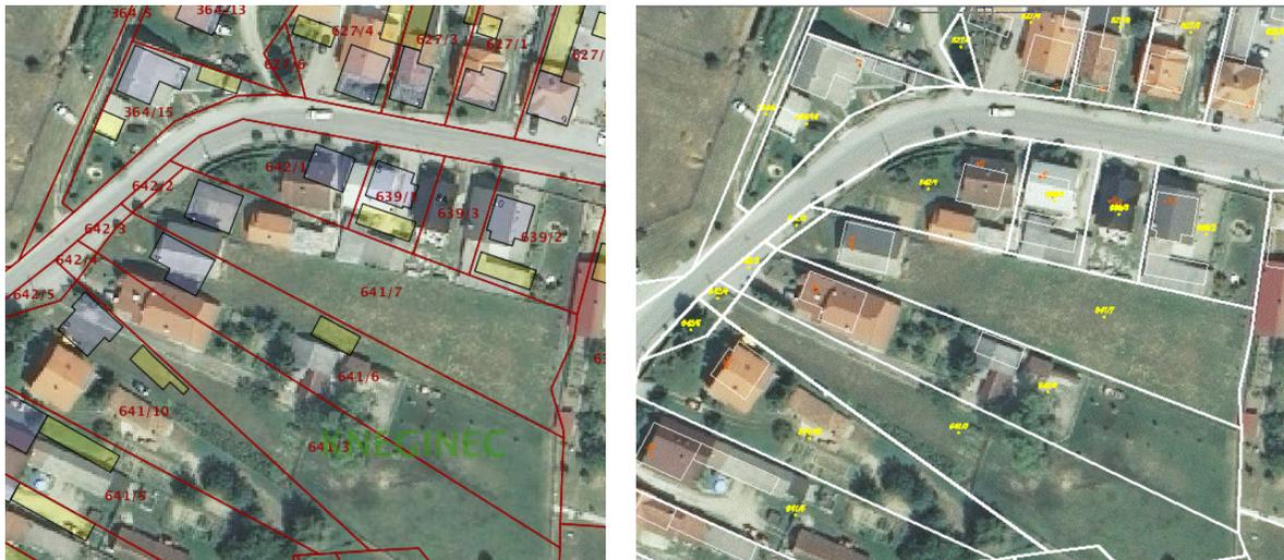
*Figure 1. DCM overlapped on DOP before and after improvement*
